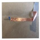
6. Place a piece of copper tape over the positive leg of the LED. Place the tape as smoothly as possible. When you get to the corner of the rectangle, instead of cutting the tape, turn the tape back on itself and then fold down towards the other direction. Complete the three sides of the positive side.
